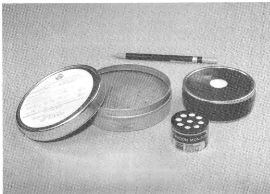
FIGURE 3.—Types of passive radon detectors. An alpha track detector (ATD, front) and two types of charcoal canisters (rear) are shown. Photo by Jim Rigby.
