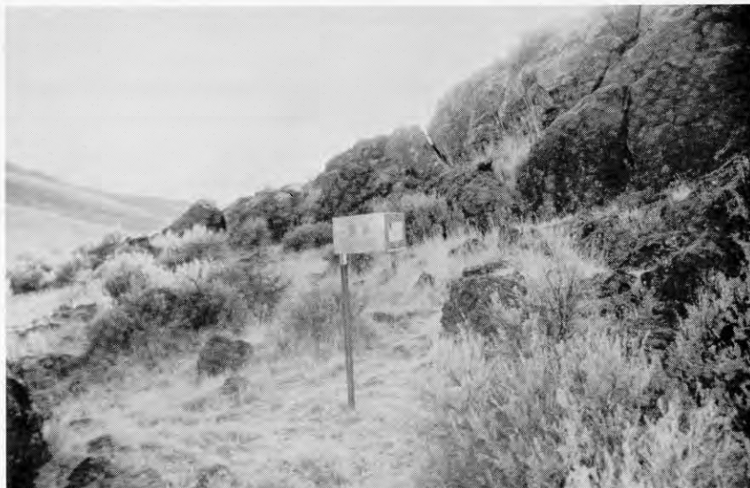
FIGURE 19.—Ventilated shelter box used to house radon detection instruments used in ambient air survey, located 1.0 m above ground level. Photo by Jim Rigby.
